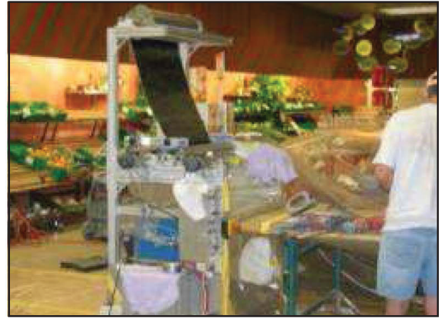
Wetting of Wrap with Saturant
