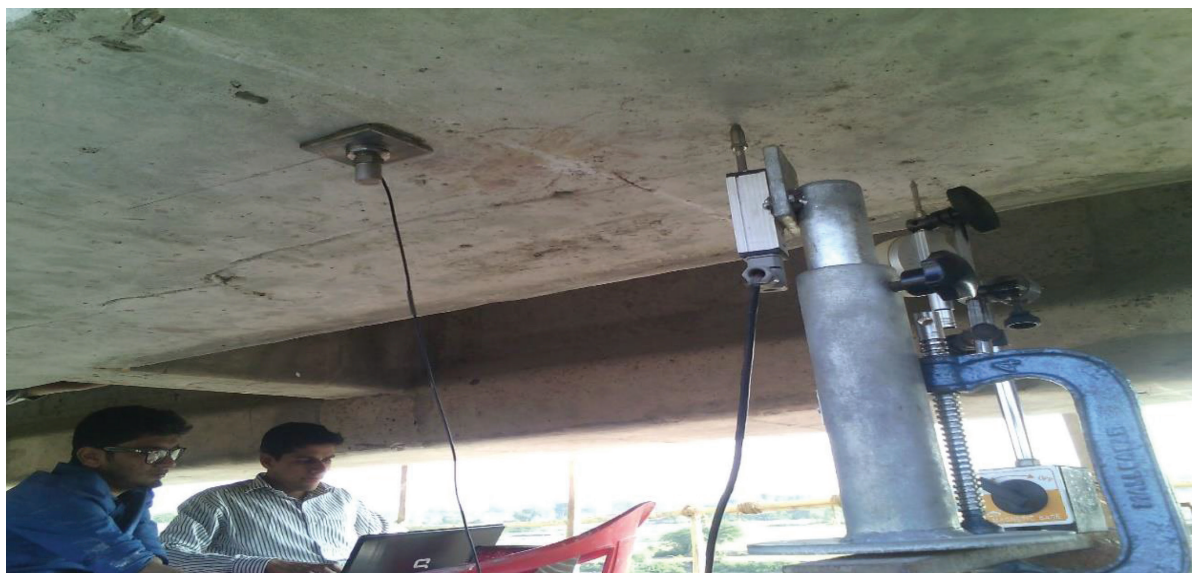
Fig 2. Structural health monitoring of Ratlam railway bridge with help of sensor
