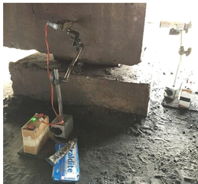
Fig.8: Placing of Linear Potentiometer
