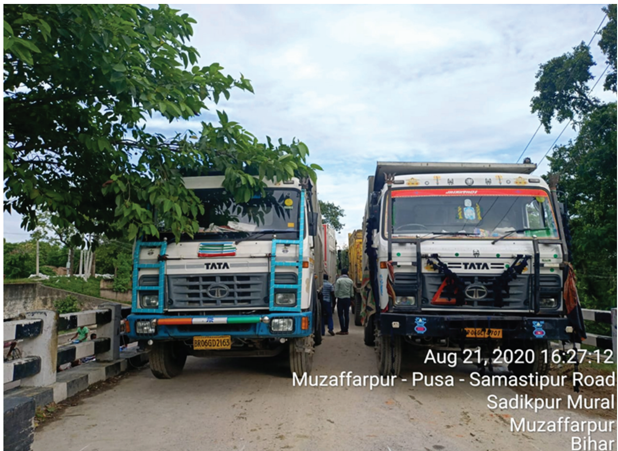
Fig 15: Loaded Trucks placed for Static Load Testing
