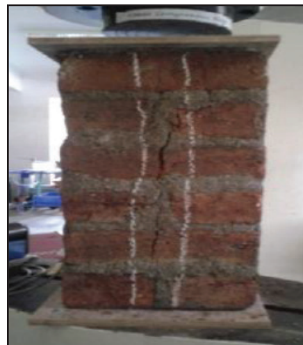
Figure 1 : Vertical Splitting Cracks
