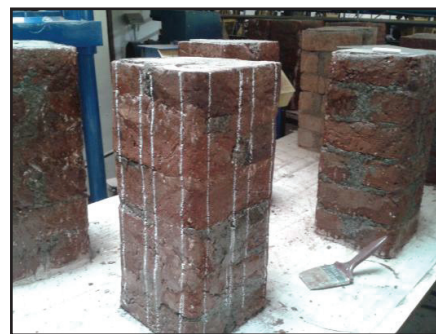
Figure 2 : Marking for FRP strips on Primer applied specimen
