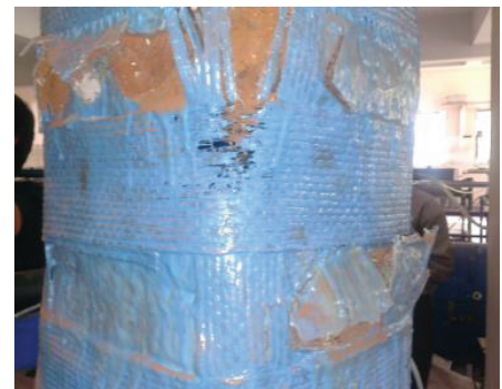
Figure : Failure of CWOA Specimen
