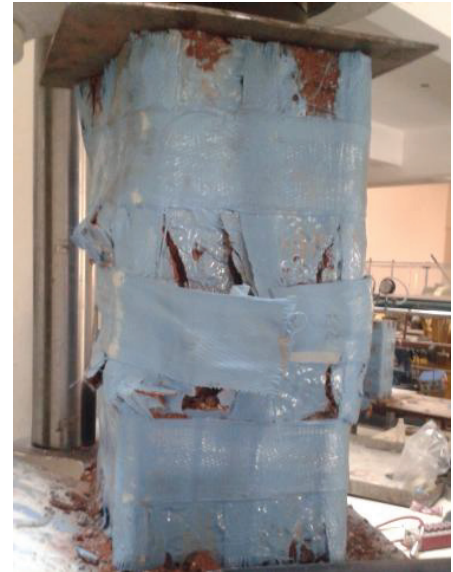
Figure 5 : Failure of GWOA Specimen
