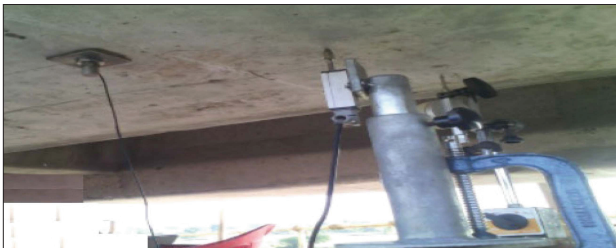
Fig. 7 Arrangement of deflection sensor and accelerometer
