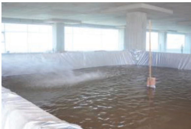
Fig. 8 Load testing on strengthened slab panel (Courtesy:- M/s R & M International Pvt Ltd)
