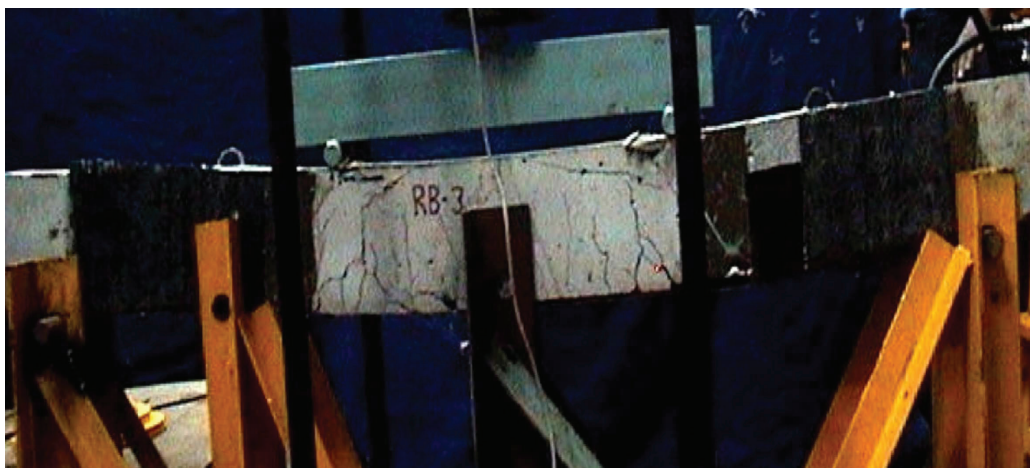
Fig. 7. Beam at failure.
