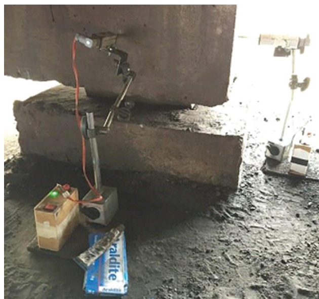
Fig.8: Placing of Linear Potentiometer
