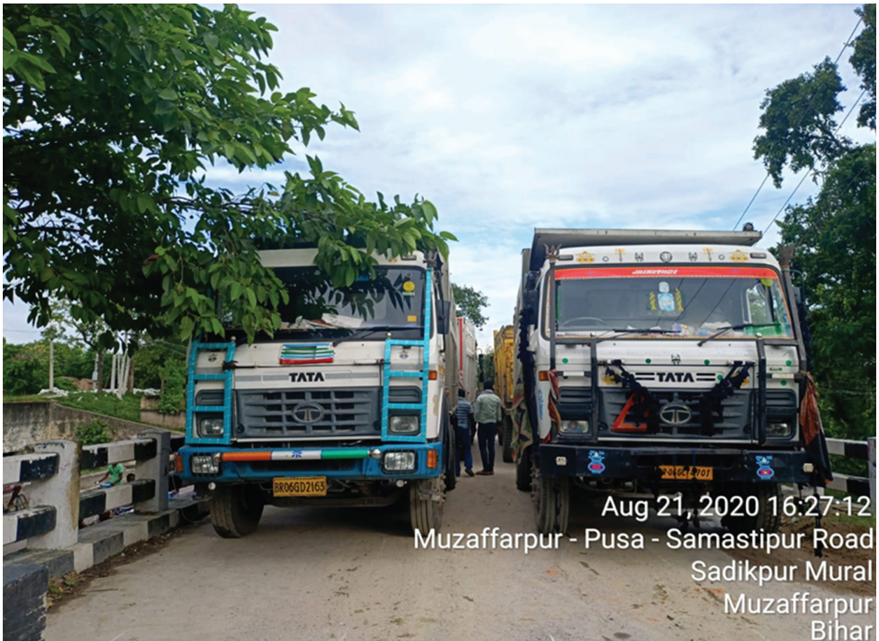
Fig 15: Loaded Trucks placed for Static Load Testing
